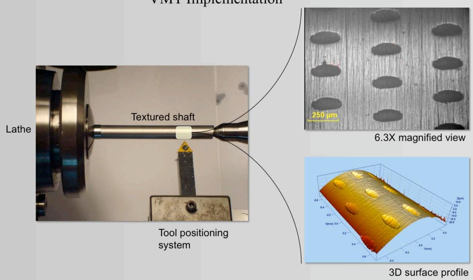
• VMT system is developed and optimized to >90% texture accuracy
