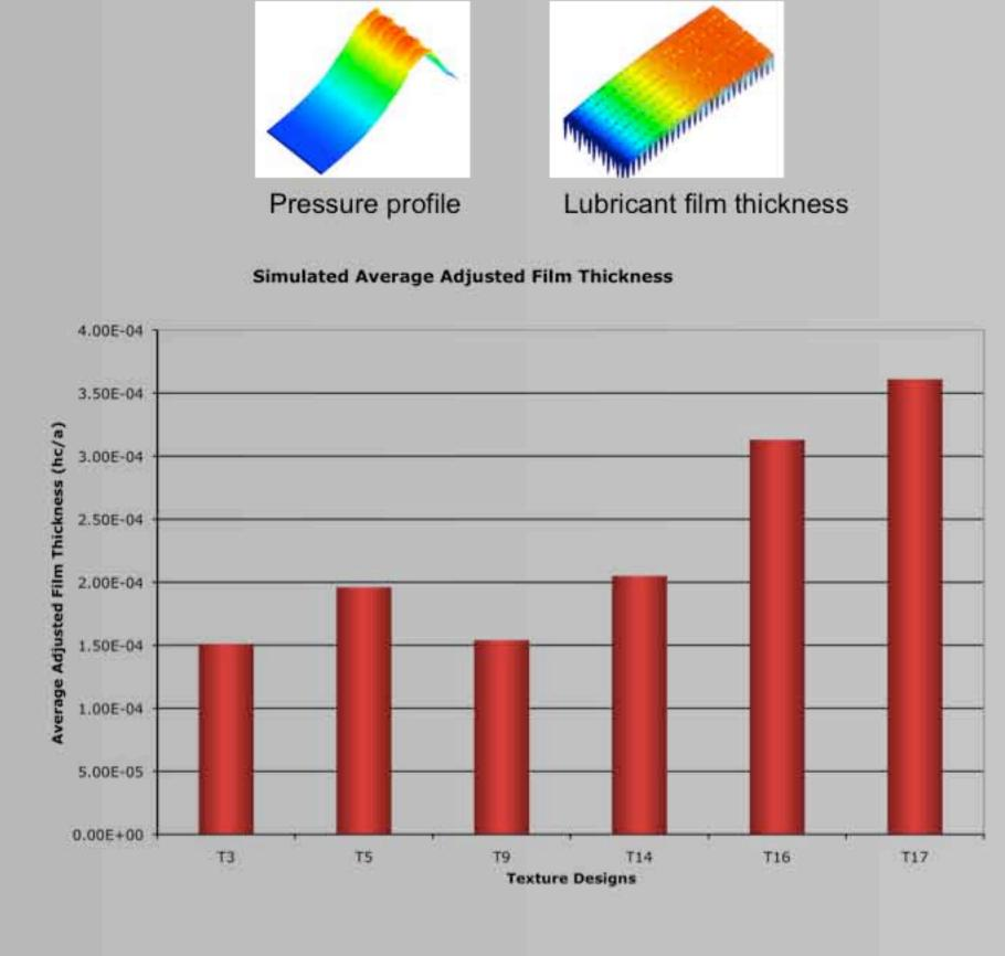
Simulation tools are used to calculate the film thickness for each texture design
